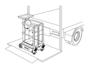
Raise the tail lift to the vehicle bed height. Unlock the castors and manoeuvre to the desired location on the vehicle and tie down as described above.
