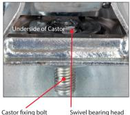
Swivel bearing head should feel free to rotate and not loose
